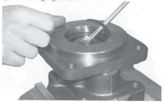
**11.**Use bearing puller to remove outboard bearing.
