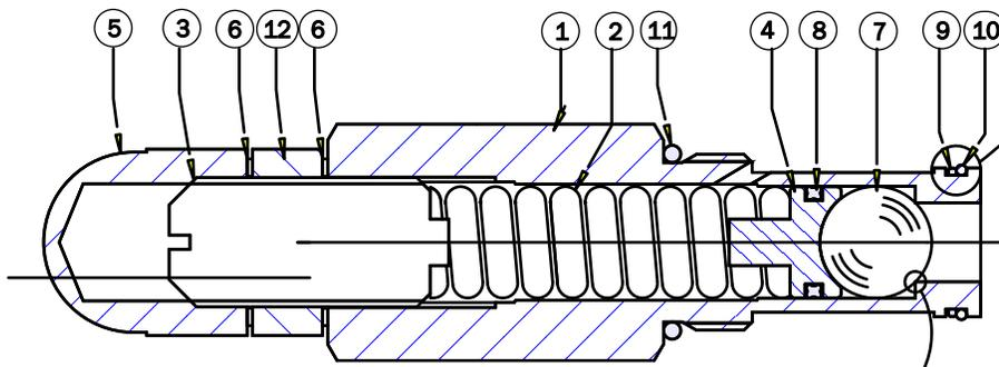
If items 9 or 10 are damaged, oil will bypass relief valve
