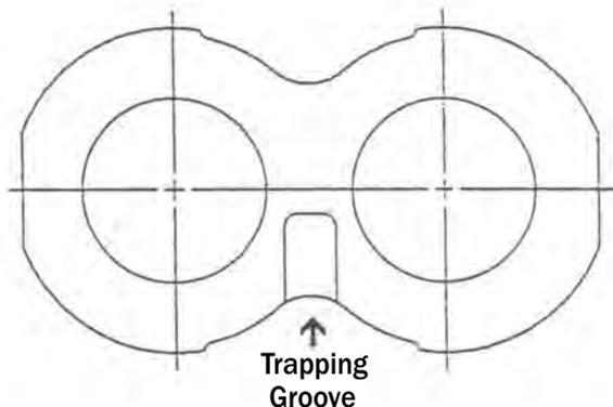
The trapping groove must be placed on the high pressure (discharge) side of the pump
