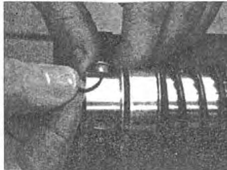
**8.** Apply a light coating of grease to quad seal ring. Slip snap ring onto clevis pin to secure it.
