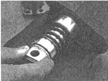
**7.** Hold opposite end of spool and push on piston assembly until piston hole lines up with hole in valve spool. Slide clevis pin into hole.
