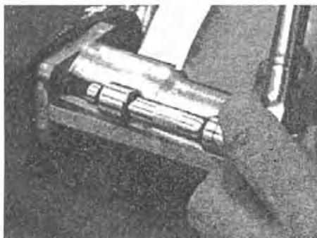
**10.** Alternating cross corners, torque cap screws to 24 ft. lbs.
