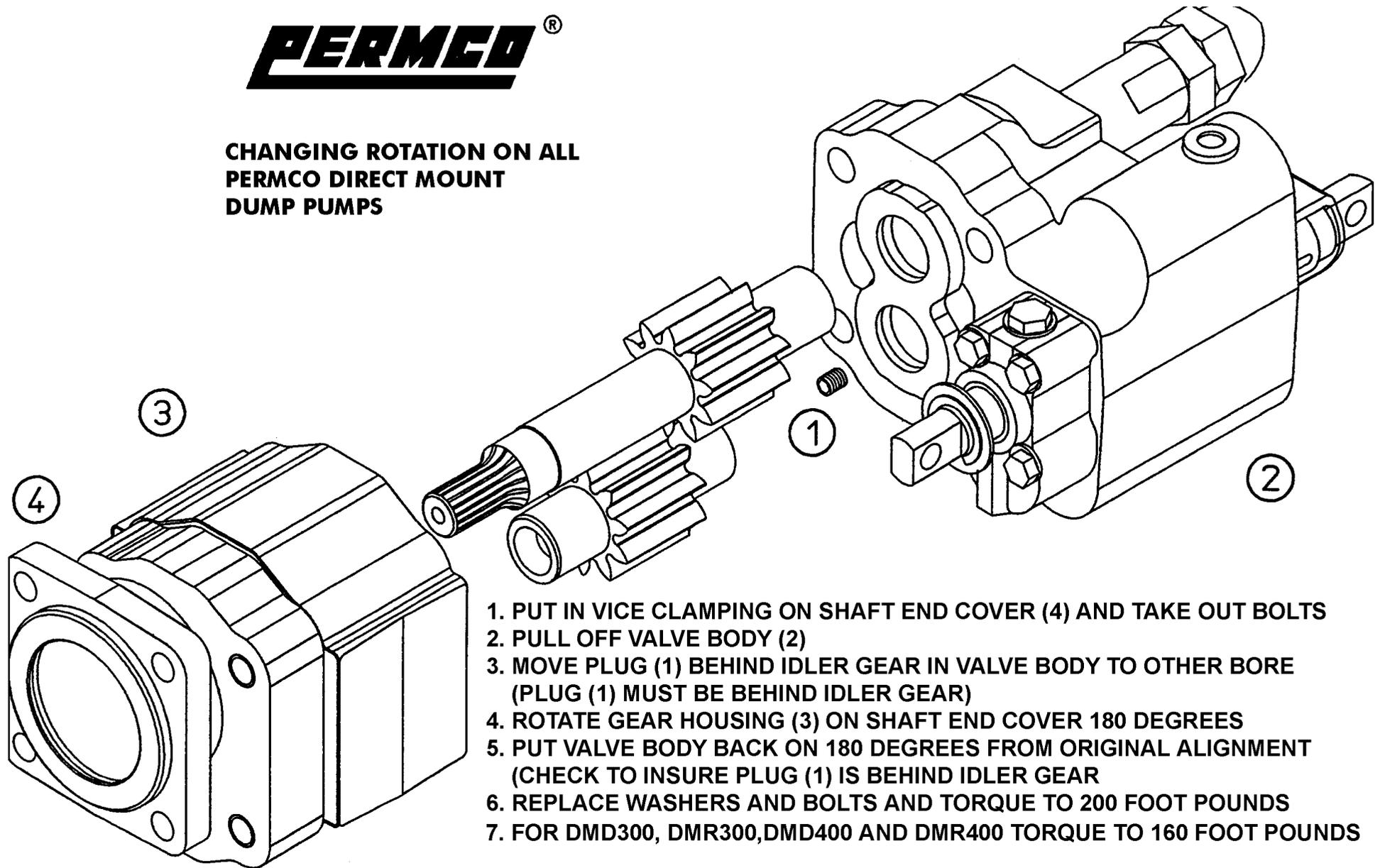
1. PUT IN VICE CLAMPING ON SHAFT END COVER (4) AND TAKE OUT BOLTS
