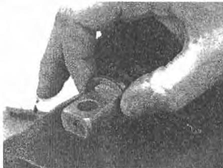
**2.** Remove retaining ring from valve spool.
