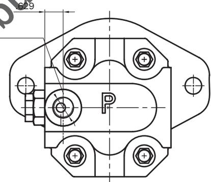
Outlet port side location available in 1/2", 5/8", 3/4", 7/8" or 1" SAE Straight Thread (ODT), SAE Split Flange, Metric Straight Thread, Metric Split Flange or BSPP (use 124 code book for port codes)
