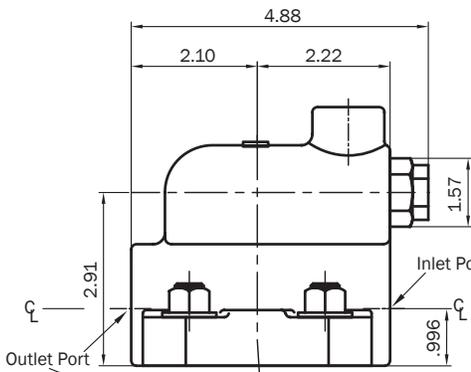
Relief valve exhaust port top location available in 3/8" or 1/2" SAE Straight Thread (ODT), Metric Straight Thread, or BSPP
