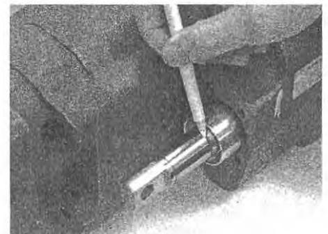
**6.** Apply light coating of grease to small O-ring and carefully place it into large detent groove in valve spool.
