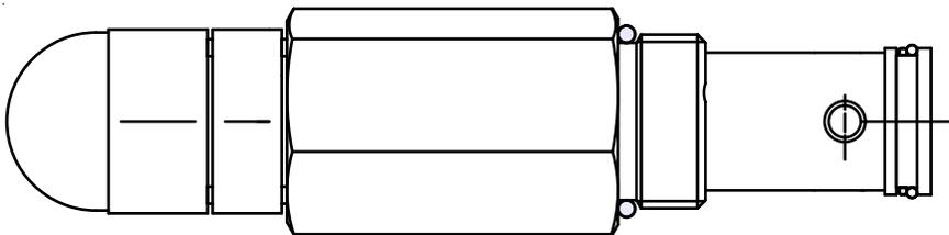
\* In the event the relief valve is disassembled - Calibration must be done on a test stand
