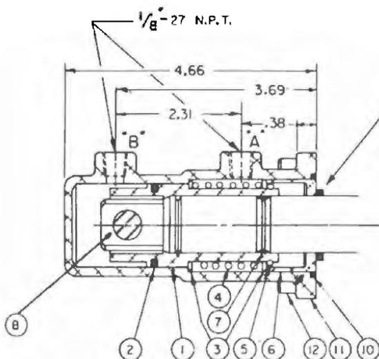
Be sure O-ring is in proper position in groove in valve housing before starting assembly.
