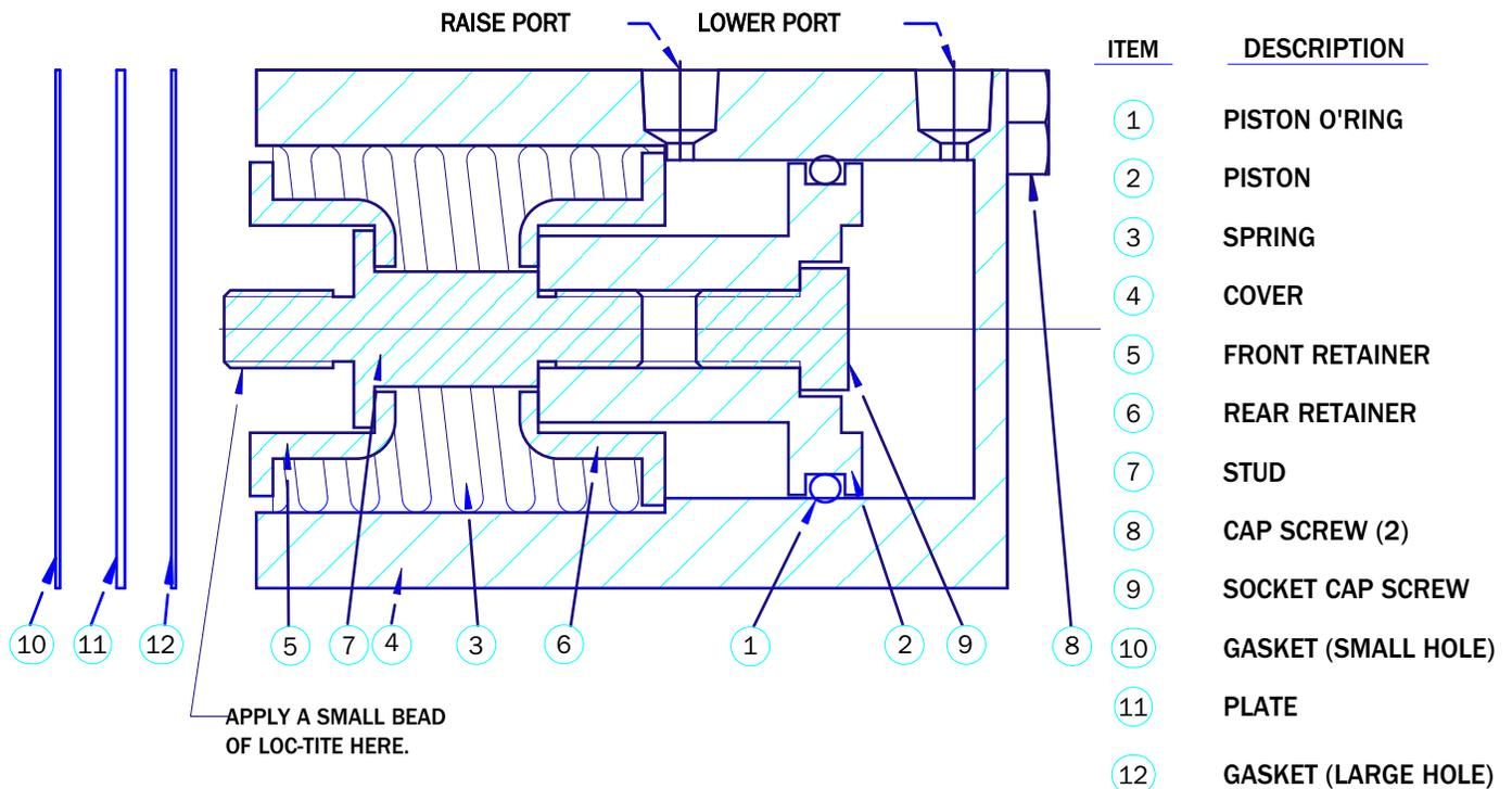
NOTE: 997-00863 ASSEMBLY DOES NOT INCLUDE THE VALVE SPOOL.
