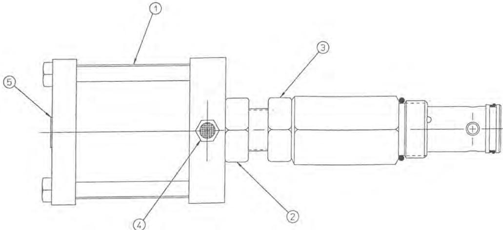
The relief valve comes preset at the factory for 2500 PSI and 3200 PSI. The lower setting is to be used for dump trailer applications and the high setting for live floor trailers. To change between the low and high setting, air pressure is induced via port 5. With a minimum of approximately 60 PSI air at this port, the relief valve setting will change to 3200 PSI. Without pressure at port 5, the unit reverts to the low-pressure setting.
